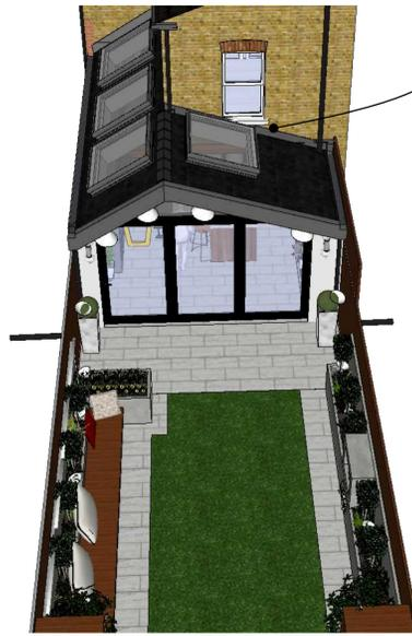
New roof is set 120mm below the existing window sill at first floor level
