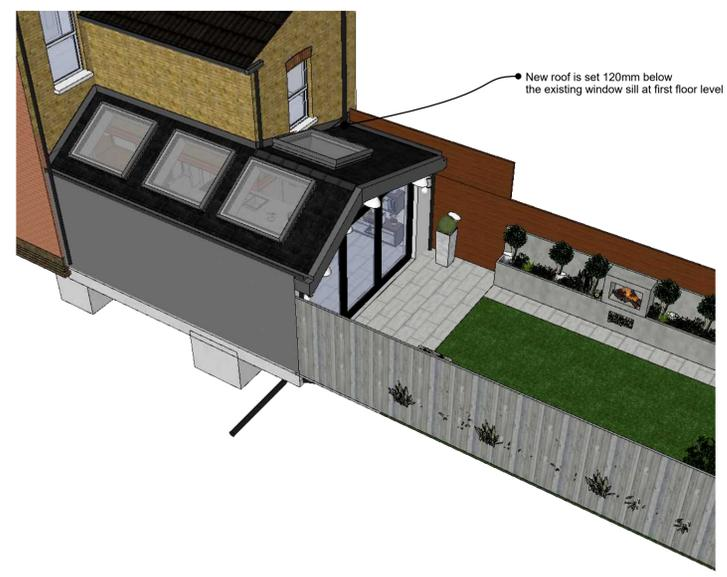
New roof is set 120mm below the existing window sill at first floor level
