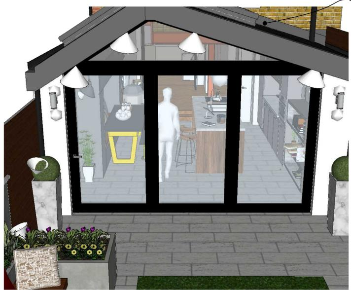
New roof is set 120mm below the existing window sill at first floor level
